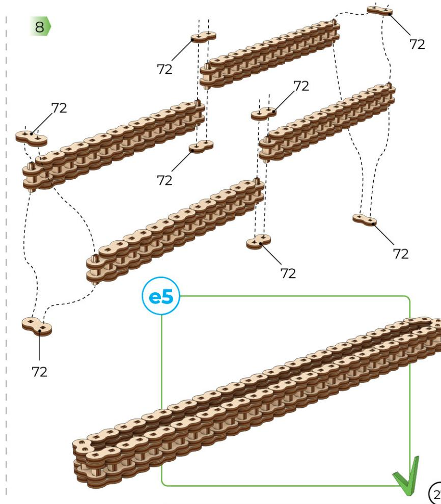
**ENG** The chain should consist of 32 links. If after assembly and aligning the length of the chain exceeds 205 mm, remove one link. If after assembly and aligning the length of the chain is less than 195 mm, align the chain so that it stretches to the required size (see diagram at the bottom of page).
