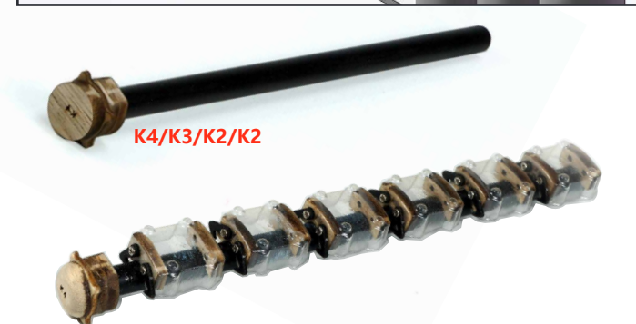
使用胶带将塑料件缠绕到18mm的圆棒上，再用热吹风加热定型。 Wrap the plastic parts onto an 18mm round bar with adhesive tape, and then heat them with hot air for shaping.
