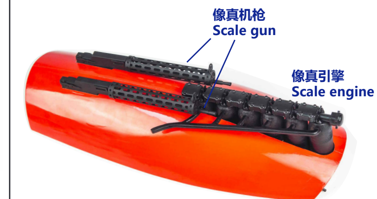
注意：像真件拼装好后， 喷黑色油漆。 Note: spray black paint after assembling the scale parts.
