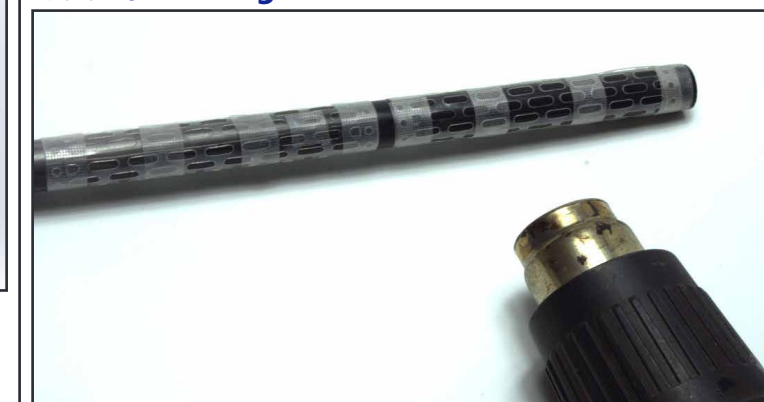
使用胶带将塑料件缠绕到18mm的圆棒上，再用热吹风加热定型。 Wrap the plastic parts onto an 18mm round bar with adhesive tape, and then heat them with hot air for shaping.
