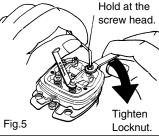
6. If clearance is correct, loosen the locknut on the other rocker-arm and repeat steps 1 to 5 above. Finally, replace rocker box cover.
