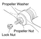
Obviously, this can be very hazardous. To eliminate such dangers, the O.S. Safety Locknut Assembly was devised. Install this as follows:
