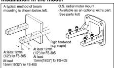
Make sure that the mounting beams are parallel and that their top surfaces are in the same plane.
