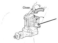
With the transmitter throttle trim lever fully retarded, adjust the throttle servo linkage so that the throttle rotor is fully closed (i.e.engine stopped) when the stick is fully retarded.
