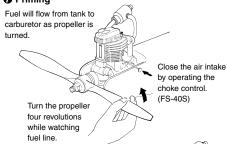
Turn the propeller 3 to 4 turns counterclockwise smartly by finger in the direction of arrow. Turn approx. 10 turns when the engine is cold.
