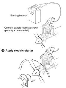
Check that the throttle is one-third open from the fully closed position. Bring the starter into contact with the spinner nut or spinner and depress the starter switch for one or two seconds. Repeat if necessary. When the engine fires, withdraw the starter immediately.
