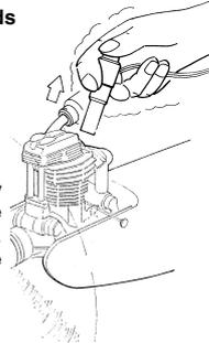
If the engine stops when battery leads are disconnected, close the needle-valve a little (approx. 45°) further, and restart the engine.
