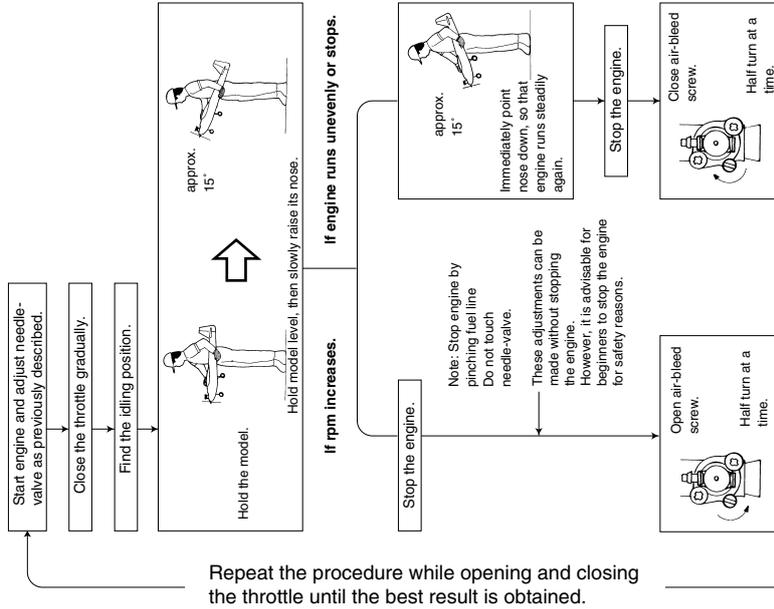
**Attention: Do not leave the glowplug connected to the battery while adjusting the carburetor throttle.**
