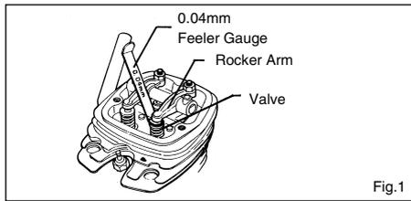
(2) If a clearance is found to be outside either of these limits, it should be reset as follows.
