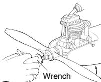
Tighten the propeller nut firmly so that compression is first felt around this position (i.e. with blades horizontal) when turning the propeller in the direction of arrow.
