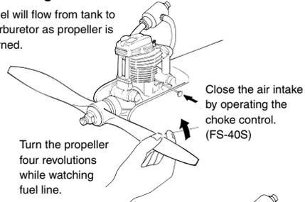
Turn the propeller four revolutions while watching fuel line.
