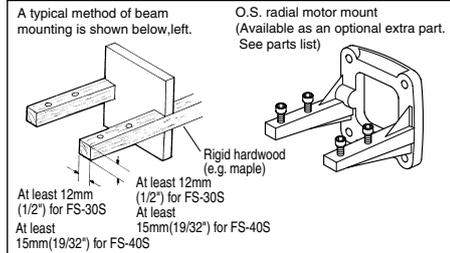
**Make sure that the mounting beams are parallel and that their top surfaces are in the same plane.**
