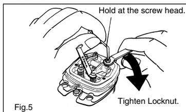
5. Remove 0.04mm feeler, rotate prop through two revolutions and recheck gap.
