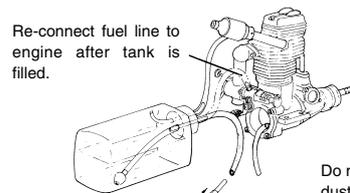
Disconnect fuel line from the fuel inlet, and connect it to the tubing from the fuel pump.
