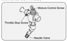
Two mixture controls are provided on this Carburetor.
