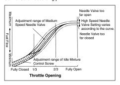
NOTE: With this carburetor, neither the Idle Mixture Control Screw adjustment, nor the Medium Speed Needle Valve adjustment will have any effect on mixture strength when the throttle is fully (or almost fully) open.
