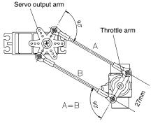
Throttle control rod A and B should be equal length. Set the linkage so that the servo output arm and throttle arm are parallel when the throttle stick on the transmitter is at middle position. If differential throttle movement is required, make necessary adjustment at the transmitter.
