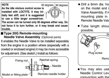
Remove the needle-valve holder from the carburetor and fit the plug screw in its place.
