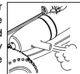
Next, disconnect the glowplug battery and try running the car on the track. If the engine stalls, open the throttle fractionally, but try to keep the engine running as rich as possible: if it stops because of being excessively over-rich, close the Needle-Valve 30° and try again.
