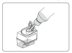
◆ At the end of each operating session, drain out any fuel that may remain in the fuel tank. Afterwards,energize the glow-plug and try to restart the engine, to burn off any fuel that may remain inside the engine. Repeat this procedure until the engine fails to fire. Do this while the engine is still warm.
