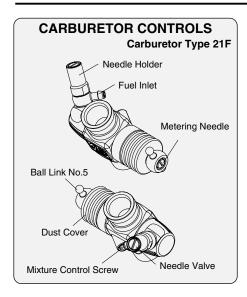
Three adjustable controls are provided on this carburetor.
