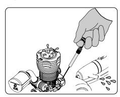
Then, inject some after-run oil into the engine, and rotate the engine with an electric starter or the recoil starter for 4 to 5 seconds to distribute the oil to all the working parts.
