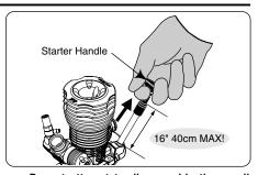
Do not attempt to disassemble the recoil starter. If you do so, the very strong spring inside will be suddenly ejected. This can be very dangerous.
