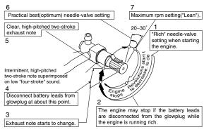
Note: Although this is a two-stroke engine it fires like a four-stroke at these rich needle-valve settings-i.e. ignition of the fuel charge takes place at every fourth stroke of the piston instead of at every second stroke.
