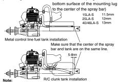
Control line models tend to receive more abrupt changes of attitude than R/C models, which results in air bubbles being drawn from the fuel tank. Pay careful attention to the plumbing and fuel tank position.
