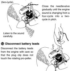
If the engine stops when battery leads are disconnected, close the needle-valve a little (approx. 45°) further, and restart the engine.
