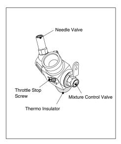
Three adjustable controls are provided on this carburetor.
