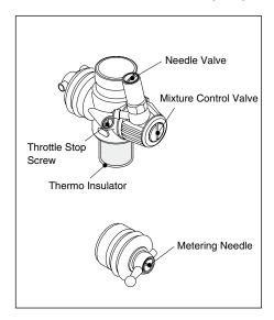
Four adjustable controls are provided on this carburetor.
