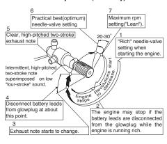
Note: Although this is a two-stroke engine it fires like a four-stroke at these rich needle-valve settings-i.e. ignition of the fuel charge takes place at every fourth stroke of the piston instead of at every second stroke.
