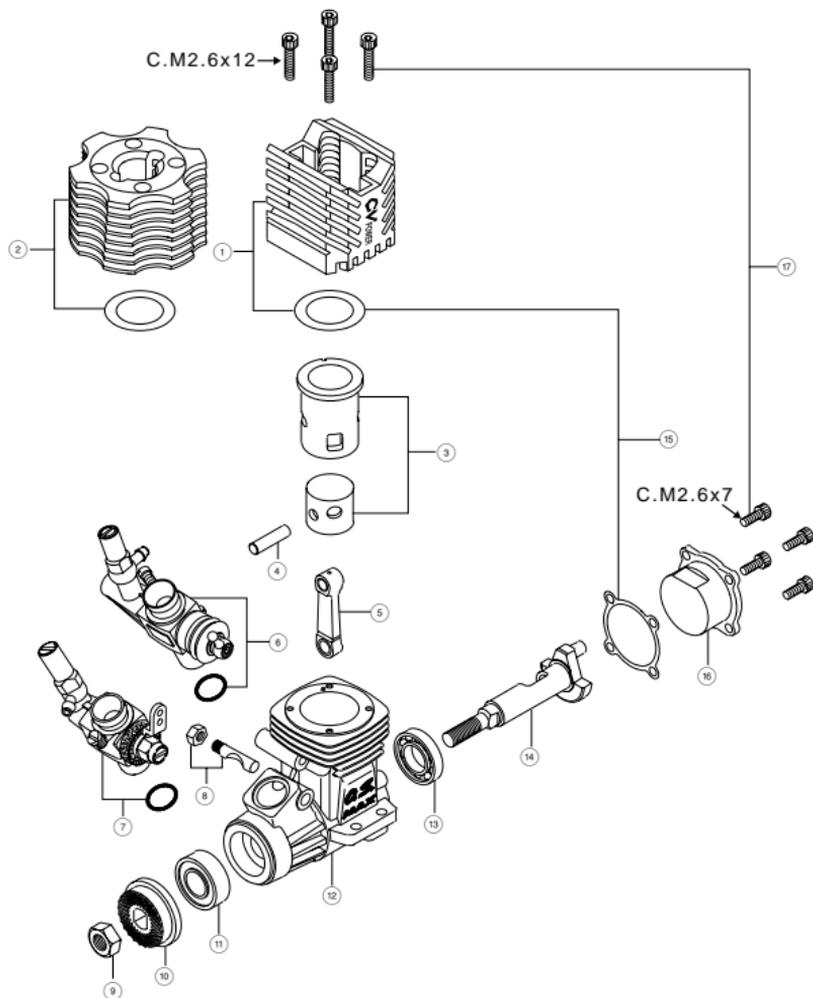
\* Type of screw C...Cap Screw M...Oval Fillister-Head Screw
