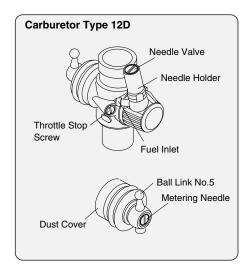
Three adjustable controls are provided on this carburetor.
