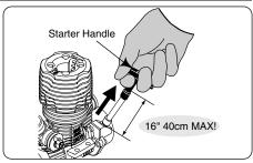
Do not attempt to disassemble the recoil starter. If you do so, the very strong spring inside will be suddenly ejected. This can be very dangerous.
