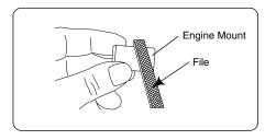
Make sure that the vehicle's engine mounting surfaces are level and in the same plane. Poor installation may cause distortion of the crankcase, bearings, etc., resulting in erratic running and loss of performance.
