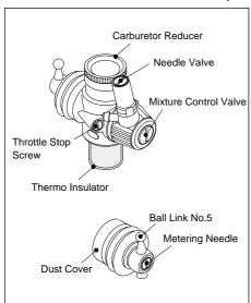
Four adjustable controls are provided on this carburetor.
