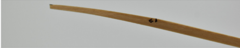
The forward part of a bevelled and edge bent plank, ready to be glued and pinned into position. The slight edge bend was simply done when the plank was damp, and bent using fingers and thumb.
