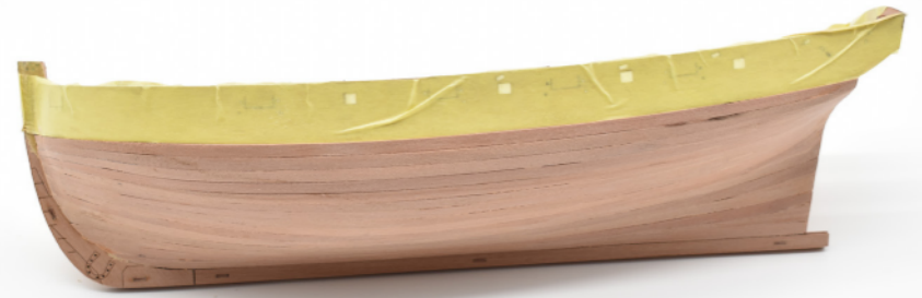
40. Second planking complete, sanded and filled. To get to this stage, several filling and sanding sessions were required. The filler used is a water based type, so it can be diluted and thinned, so it is able to flow into every gap. Before the sanding and filling process started, the engraved upper bulwark pattern area and the areas not to be painted white were masked off, as can be seen.
