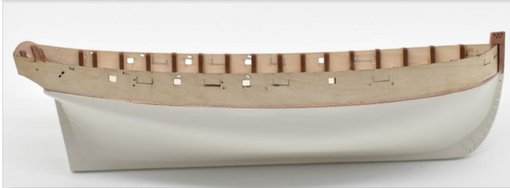
46. Hull painting fully complete and all masking removed. Touch up any areas that require attention
