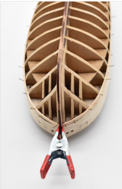
The first plank successfully pinned and glued in place.
