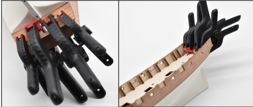
49. The outer lower stern counter can now be added (41) Brush glue watered down PVA wood glue to the contact surface and clamp in place as shown
