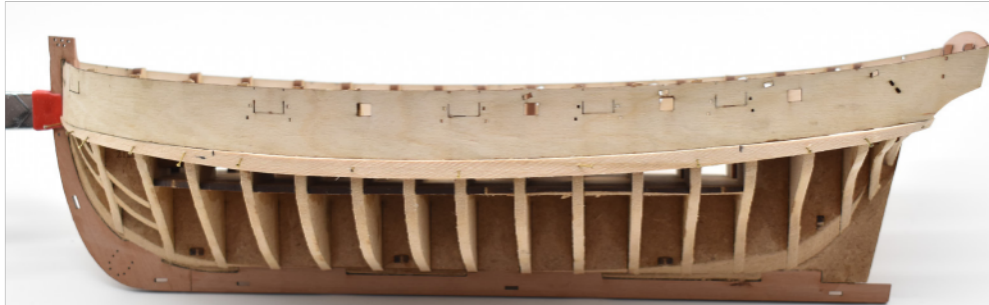
The forward part of a bevelled and edge bent plank, ready to be glued and pinned into position. The slight edge bend was simply done when the plank was damp, and bent using fingers and thumb.
