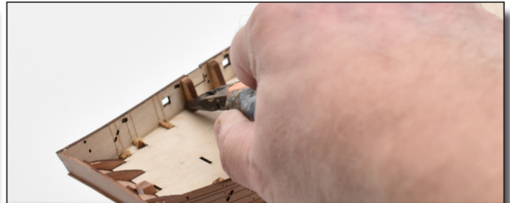
53. Remove all bulkhead tabs above deck level by carefully bending and twisting with a pair of pliers or similar. Once removed, sand any remaining stubs flush with the deck.
