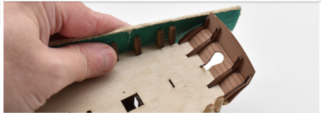
22. Sand the side bulwark tabs and stern counter and transom so that the run of the pre cut bulwark parts run nice and smoothly.
