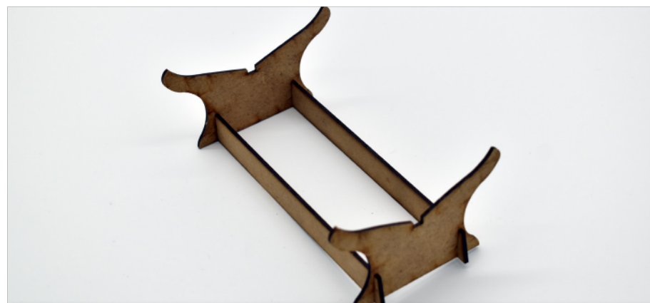
50. Make up the build cradle using parts 26, 27 and 28. It can be glued using PVA wood glue. This is only a temporary stand until the model is almost complete. (The final stand may look different to the one shown above)
