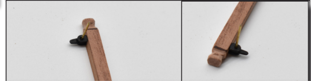
Glue the pawl brackets (PE-12) into each slot in 114. Insert the pawl (PE-13) and then lock it in place with a brass pin, which is then glued at the end and the excess snipped off.
