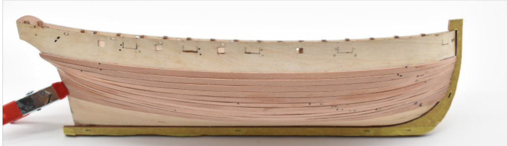
Planking progress with 12 planks per side done. Some stern planking is clamped to ensure they are fully adhered to the hull.
