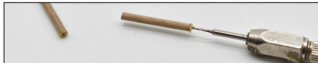
Above - using cyano glue, fix the cap (PE-17) to the top of each 25mm length of dowel, and then drill a 0.8mm hole through the hole in PE-17 and into the centre of the dowel.
