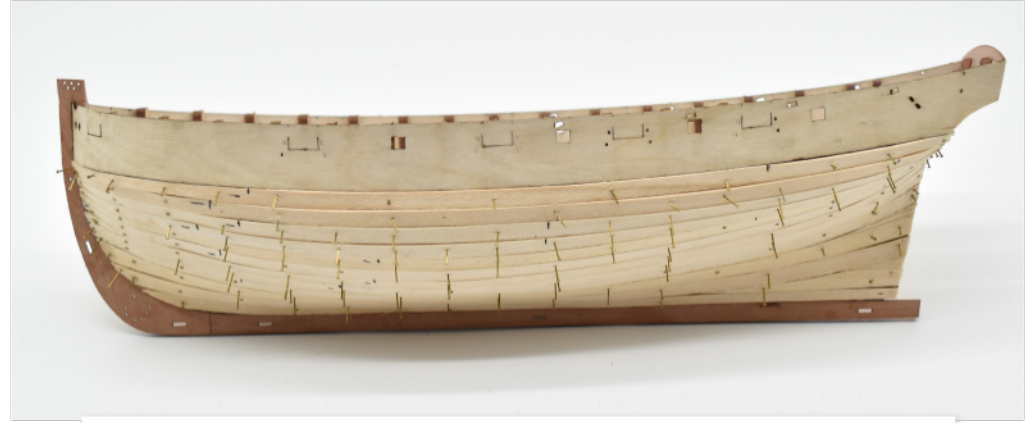
First planking complete. There are 12 planks per side, with a few 'Stealers' at the stern.
