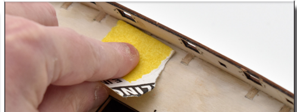
53. Remove all bulkhead tabs above deck level by carefully bending and twisting with a pair of pliers or similar. Once removed, sand any remaining stubs flush with the deck.
