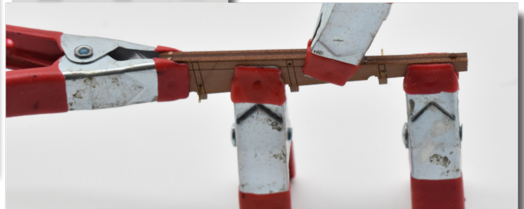
41. Make up the stern using part 59 for the core, and 82R (right) and 82L (left) glued to each side of part 59, with an alignment peg (65). Use PVA wood glue and clamp together until cured.
