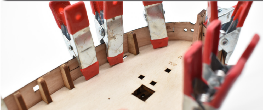
29. The bulwarks were clamped at many bulkhead stations for the prototype. Once in place, leave to thoroughly cure for 24 hours and then remove all clamps, as shown below.
