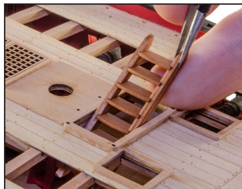
622. Glue the ladder into position through the quarterdeck coaming as shown.
