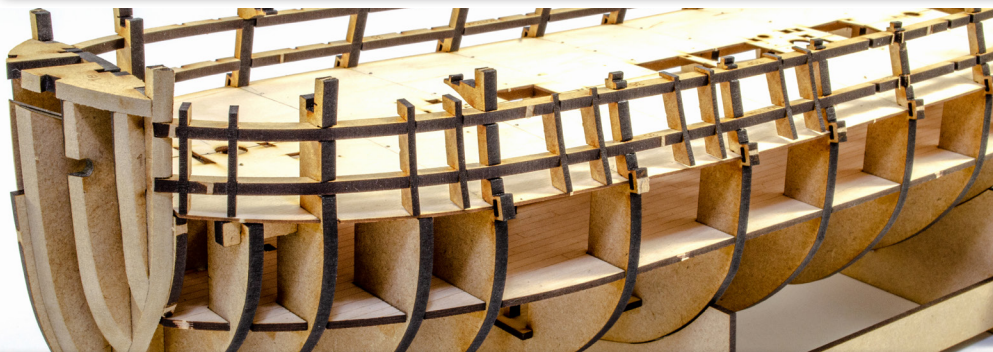
78. The Vertical Gun Port Frames glue into the slots between the upper and lower longitudinal gun port strips.
