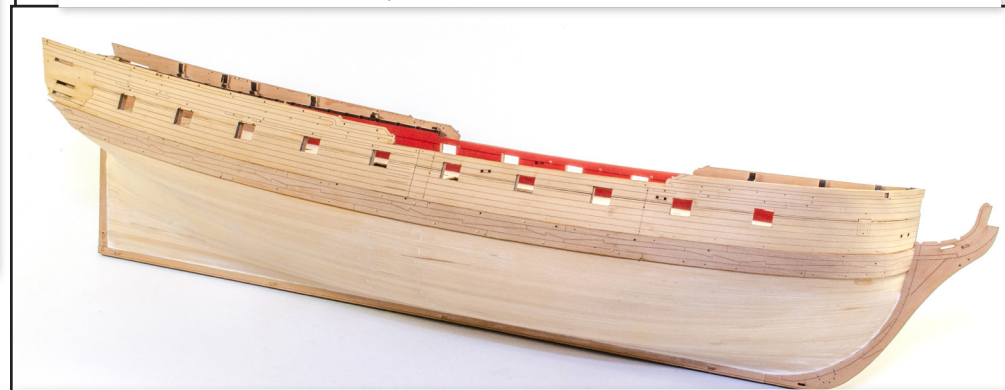
190. Both wales are now glued to the model. We used PVA for this and pinned where appropriate. There are small nail holes in the wales (NOT the larger scupper holes!), that you can use to pin. Also feel free to pin wherever you feel it necessary.
