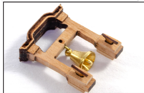
596. Cut short and glue the bent pin into the hole you just made, to hang the bell. You can either leave the belfry in natural wood or paint it black. We have chosen to paint it.
