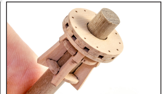
467. Glue the Capstan Upper Drum Head – Gun Deck (253) on top of your assembly as shown.
