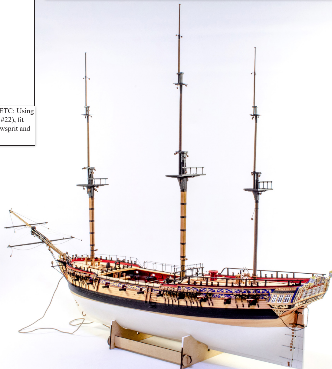
893. FITTING THE MASTS: This is quite simple, but vital you very everything properly aligned. Things should be aligned nigh on perfectly anyway, but if you need to make any adjustments to the central path of the masts, do so with a small file to the mast opening in deck, and preferably to the hole on the main deck so you don't elongate the mast base parts.
