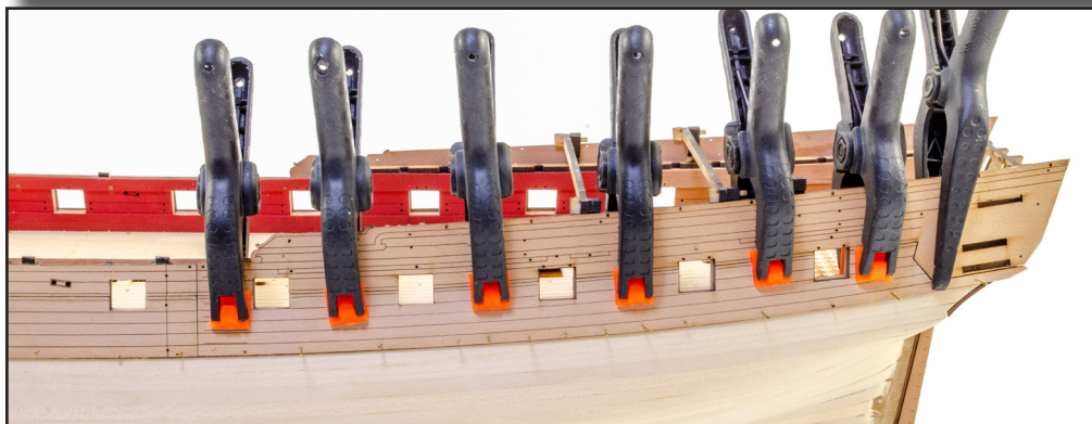
172. These can now be glued into position like the others, with clamps and also pins used along the lower edge to hold things down. NOTE: These lower pattern parts are optional. Extra pear planking is supplied in case you wish to plank this area traditionally.
