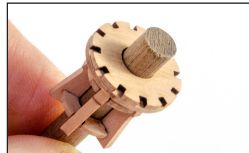
466. Now glue the Capstan Drum Head for Bars (252) into position.
