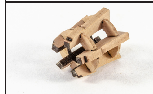
464. Glue the five capstan whelps (437), onto the two Capstan Chocks (250). You can temporarily slide the down into the chocks to help you get the shape correct.
