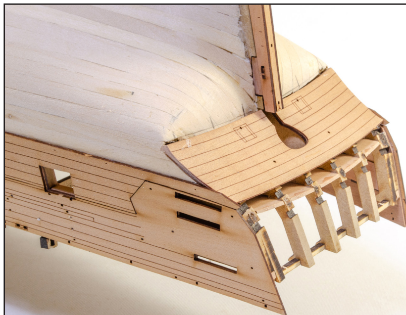
174. Before the hull can be planked, it's time to fit the Stern Lower Counter Pattern – Outer (76) from the 0.6mm wood sheet. You can curve this first if you wish, but we feel this part is thin enough to easily be glued into place over the inner pattern.
