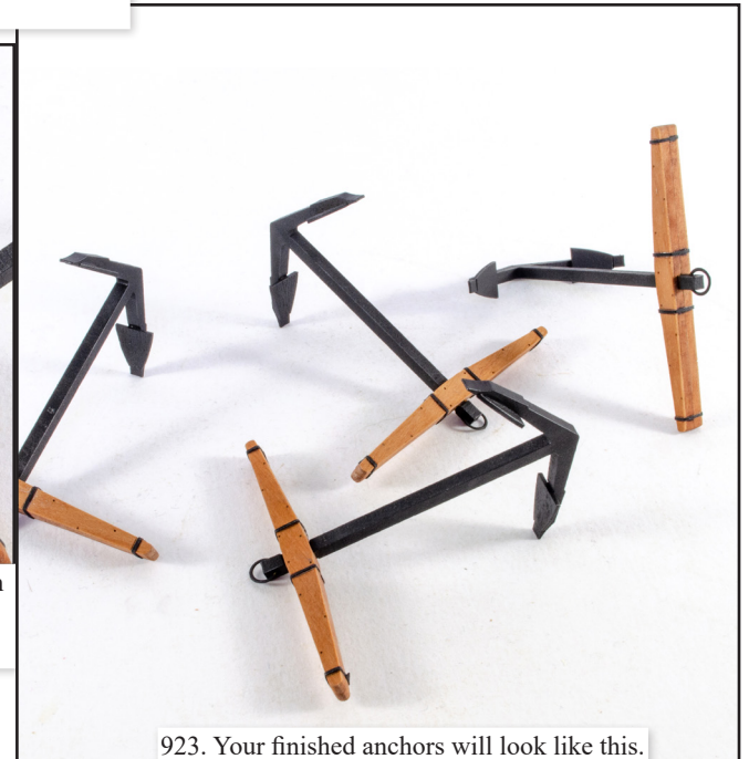
922. Use some brass wire to form the anchor hoops. Fit these to the anchors and paint black.
